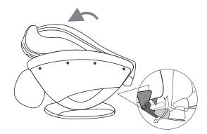
Press the " )" button on control panel turn off power on control panel and turn off the power on the switch located on the underside of the left armrest and unplug the power cord from the wall outlet. Press down the backrest folding latch located on the underside of the backrest and gently push the backrest forward (as shown in picture).
