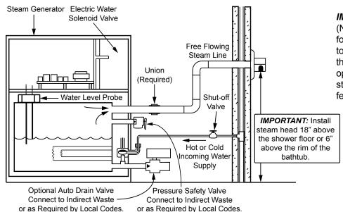
**IMPORTANT:** An optional steam diffuser (Not Included) is strongly recommended for small steam rooms. This option helps to better diffuse the steam and makes the steambath more comfortable. This option may not be necessary in larger steam rooms where the bather is sitting a few feet away from the steamhead.
