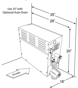
Select a location for mounting the Steam Generator that is accessible for installation and service. The access requirement indicates the minimum space for convenient access to Steam Generator.
