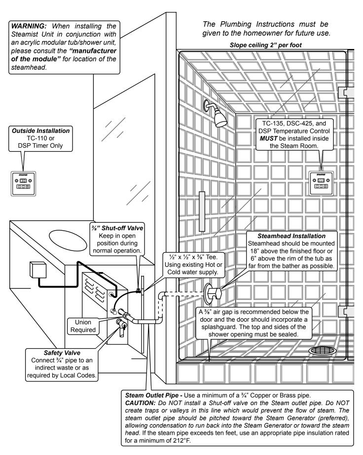
Figure 3: Typical installation
