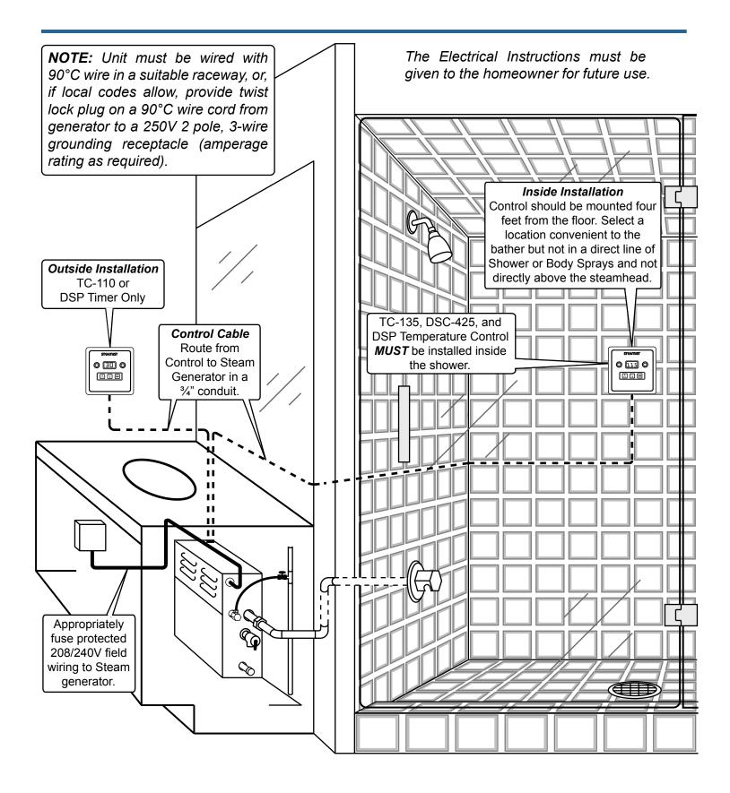
**IMPORTANT:** Run the Control Cable through a <sup>3</sup>/<sub>4</sub>" conduit. Remove protective cap when making the final connection to Control.
