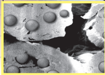
Outlast® Thermocules™ under the microscope
