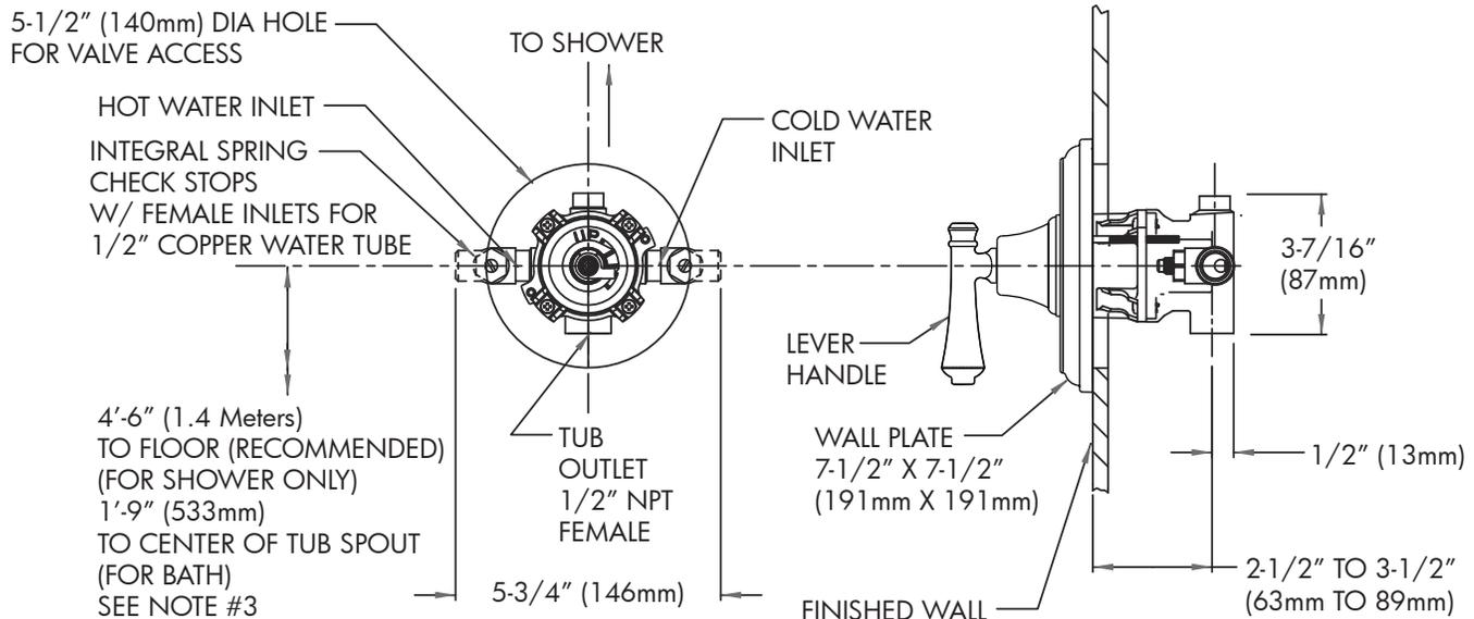
NOTE: 1. All dimensions are in inches (millimeters) unless otherwise specified and are subject to change without notice. 2. Unless otherwise specified, all inlets and outlets are 1/2" female copper sweat. 3. For ADA mounting locations, consult ADAAG, ANSI A117.1, or static regulations
