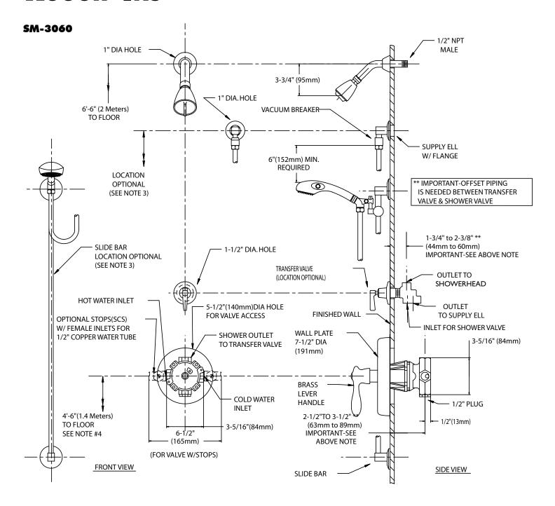
NOTE: Unless otherwise specified, all inlets and outlets are 1/2" NPTF. The location of the slide bar and supply ell is optional, but restricted by the 69" hose length running from supply ell connection to hand shower and the 6" minimum requirement between the in-line vacuum breaker and top of hand shower. Unless otherwise specified, all dimensions are in inches and are subject to change without notice. For ADA mounting locations consult ADAAG, ANSI A117.1, or state regulations.
