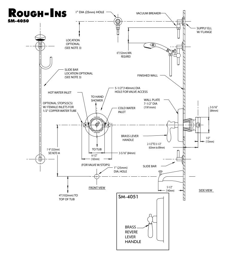
NOTE: Unless otherwise specified, all inlets and outlets are 1/2" NPTF. Locations of shower hangers are optional, but restricted by 69" hose length running from shower arm diverter connection to hand shower. Unless otherwise specified, all dimensions are in inches and are subject to change without notice. For ADA mounting locations consult ADAAG, ANSI A117.1, or state regulations.
