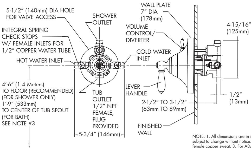
NOTE: 1. All dimensions are in inches (millimeters) unless otherwise specified and are subject to change without notice. 2. Unless otherwise specified, all inlets and outlets are 1/2" female copper sweat. 3. For ADA mounting locations, consult ADAAG, ANSI A117.1, or static regulations
