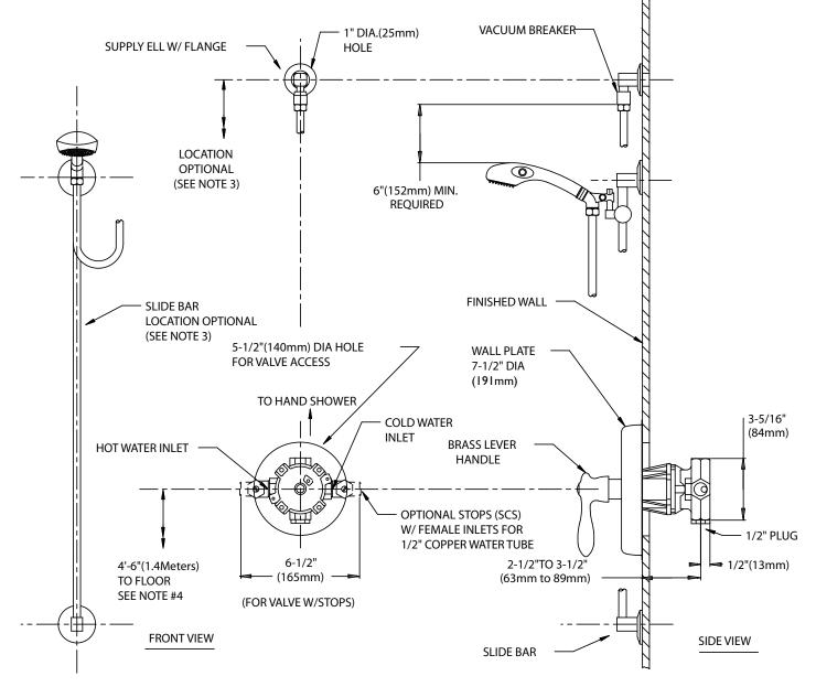
NOTE: Unless otherwise specified, all inlets and outlets are 1/2" NPTF. The location of the slide bar and supply ell is optional, but restricted by the 69" hose lenth running from supply ell connection to hand shower and the 6" minimum requirement between the in-line vacuum breaker and top of hand shower. Unless otherwise specified, all dimensions are in inches and are subject to change without notice. For ADA mounting locations consult ADAAG, ANSI A117.1, or state regulations.
