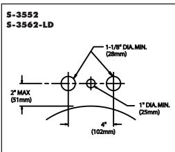
NOTE: All dimensions are in inches (millimeters) unless otherwise specified and are subject to change without notice. Lavatory inlets are sized for coupling connections. Unless otherwise specified, all inlets are 1/2" NPSM.
