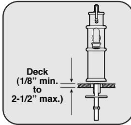
**Note:** 1/8" deck thickness only applies for stainless or composite counter tops (granite or corian, etc.)
