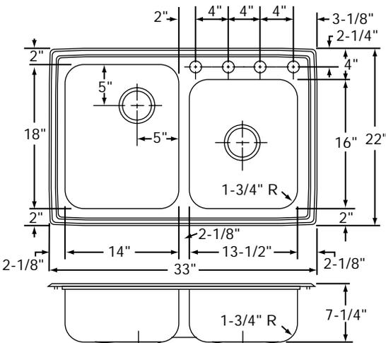
**HOLE DRILLING CONFIGURATIONS**
