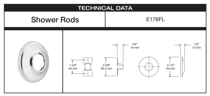
MATERIALS: Flanges are galvanized steel hanger type with concealed screw type 430 polished stainless steel covers.
