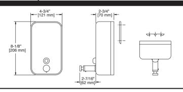
MATERIALS: Unit is fabricated 20 gauge type 304 satin stainless steel. Body dispenser
