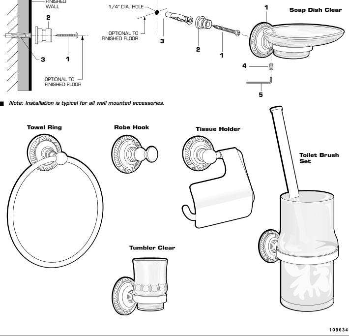
The wall mounted accessories work best if secured to a wall stud or cross brace within the wall, using the SCREW (1) supplied.
