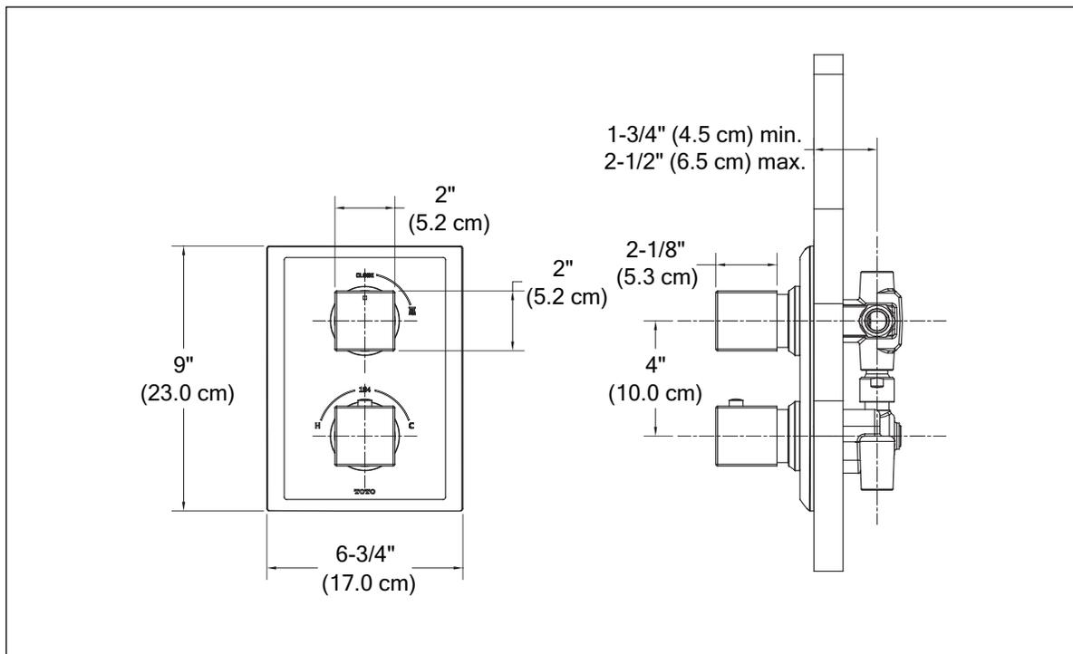
TS930C - Lloyd® Thermostatic Mixing Valve Trim with Single Volume Control
