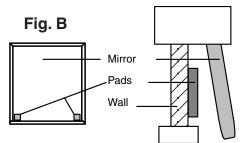
Tilt the bottom of the mirror slightly so that the pads can be placed within 1/2" to 1" of the bottom and side.
