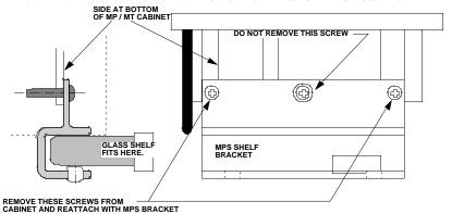
2. BE SURE THE OPEN SIDE OF THE BRACKET FACES THE MPM / MTM MIRROR. INSTALL THE CABINET, (LIGHT IF USED) AND SIDE KIT AS PER C ABOVE.
