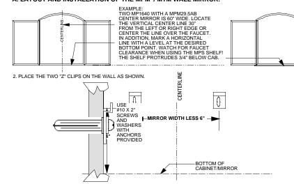
3. TEST FIT THE MIRROR. ADJUST CLIPS IF NECESSARY. WITH A PENCIL, MARK THE LEFT AND RIGHT EDGES OF THE MIRROR. REMOVE THE MIRROR WHILE INSTALLING THE CABINETS. BE CAREFUL NOT TO CHIP THE EDGES.
