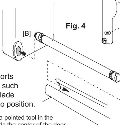
Note: To remove pins, use a pointed tool in the groove, push the pin towards the center of the door.
