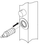
4 Press the button on the head and put on the head as below ensuring the screw hole pointing to the front
