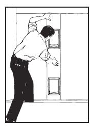
Apply 1/8" bead of adhesive to the back of the center panel, keeping the adhesive at least one inch from the tape and panel edges. Remove backing from factory applied pressure sensitive tape.
