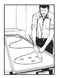
**9.** Apply a 1/8" bead of adhesive to the back of the panel, keeping the adhesive at least one inch from the tape and panel edges.
