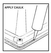
6. Apply a bead of caulk (not included) to the underside of the sink flange and position sink into counter top opening.
