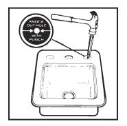
5. Fixture hole locations are identified with a gray label indicating the most desired placement. Position a chisel on the desired dot and strike with a hammer to break out the hole. Clean out fixture hole with a knife.
