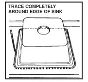
1. If it is necessary to cut out the counter top, invert sink and position onto the counter top. Locate sink front to rear and so that the bowl will not interfere with the cabinets below. Trace a pencil line around the outside edge of the sink and remove the sink from the counter top.
