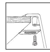
7. Attach four (4) sink clips to underside of sink. Sink clips provided will accommodate a counter top up to 1-1/2" thick. Tighten screws in front then rear first. Work from side to side. Do not overtighten. Clean up excess caulk.
