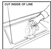
4. Using a saber saw, cut inside of cutout line. Trial fit sink to check proper fit.
