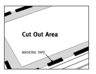
**1.** Cut out the inside of the template. Locate the template front to rear and right to left on the countertop. Make sure that the bowl location will not interfere with the cabinet below or the plumbing. Attach the template to the countertop with masking tape and draw a pencil line around the inside of the template.
