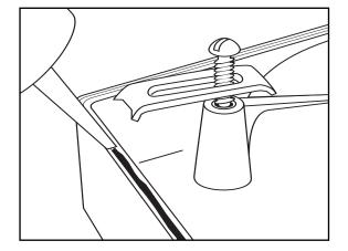
**4.** For final fit, apply a bead of caulk (not included) to the underside of the sink flange and position onto the countertop opening. First, tighten screws in front, and then tighten rear screws.
