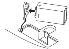
3 Tuck the battery back into the battery compartment and replace the battery cover.
