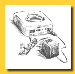
STEP 1: Plug phone cord and power cord (AC Adapter) into the back of the base. Give power cord a half turn to the right to lock in place.
