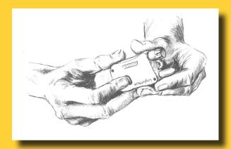
STEP 3: Run a full system check to make sure unit is working. Press the grey button on the back of the pendant and hold for <u>four full seconds</u>. Unit will beep, and after a few seconds you should hear a dial tone and the announcement "All systems are ok."
