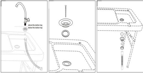
To assemble Faucet & Drain: Connect the 3/4 inch Female Hose end to the faucet end. Connect the 1 Inch Female End to a standard Garden Hose.
