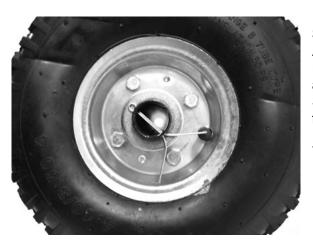
**Step 8:** Place a Wheel (G) over the end of the Axle Assembly (B) stub. Be sure air fill valve is facing outward. Place a large wheel washer (12) over Axle Assembly (B) stub, and insert the cotter pin (11) through the pre-drilled holes. Spread the ends of the cotter pin (11) to prevent the wheel from slipping off the axel (as seen in the photo to the left). Repeat the procedure for the remaining axle stub and wheel. Your Trailer Dolly is now fully assembled and ready for use.
