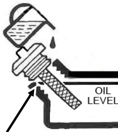
Figure 2 - Add Oil To TOP Of Threads
