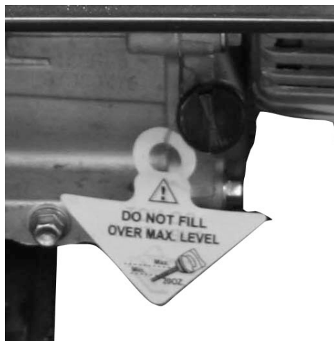
Figure 1 – Unscrew Dipstick Cap
