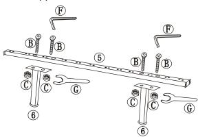
Setep 3 Fixing Side rails and Centre support bar to Headboard & Footboard.
