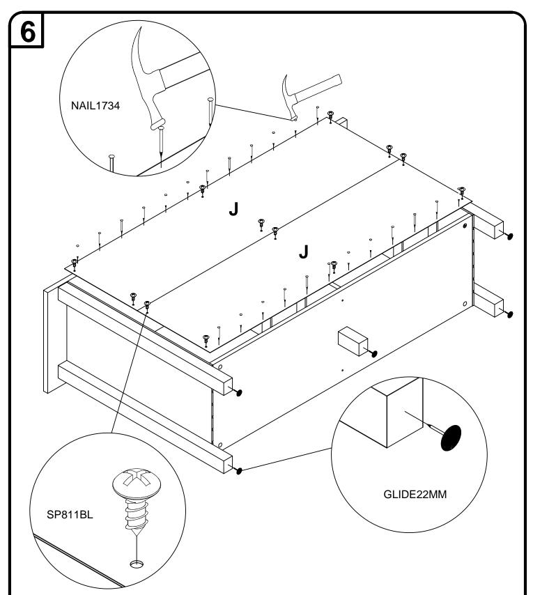
Place the unit face down. Align the Back Panel (J) over the of the unit. Make sure the assembly is square and leave equal amount of margin all around. Secure the panel by screwing 6 screws through the pre-drilled holes for both panels (2 screws on both ends and 2 screws in the center). Next, nail the top and bottom (as shown above) with approximately 4" spacing between the nails. Make sure to keep the nails centered on the edges to avoid splitting of the boards.
