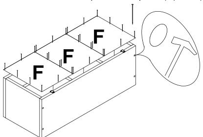
Insert the cover caps into the heads of the exposed wood screws on the top and bottom. Gently tap them into place using a hammer.
