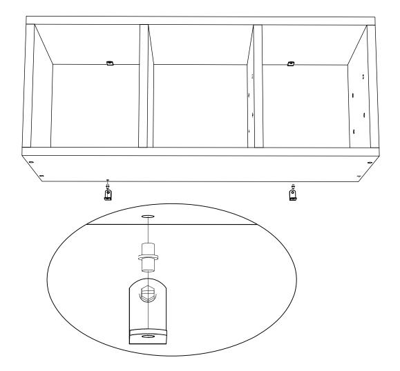
Place the unit in desired position, mark the positions of the angle brackets by tapping a nail or awl through the holes in the brackets into the wall. Then, remove the nail or awl. Attach the angle brackets using the washer head screws provided, for the most secure attachment drive the screws into the wall studs. If it cannot be utilized, use the self-drilling drywall anchors, included in this package. Follow these instructions.
