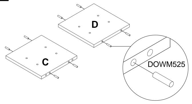
NOTE: Make sure the metal pin go in as far possible, they should stick out no more than  $\frac{3}{8}$  of an inch.
