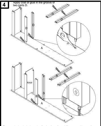
Turn camlocks clockwise using flat (preferred) or phillips screwdriver until full stop(slightly over  $\frac{1}{2}$  a turn to lock the bolt)
