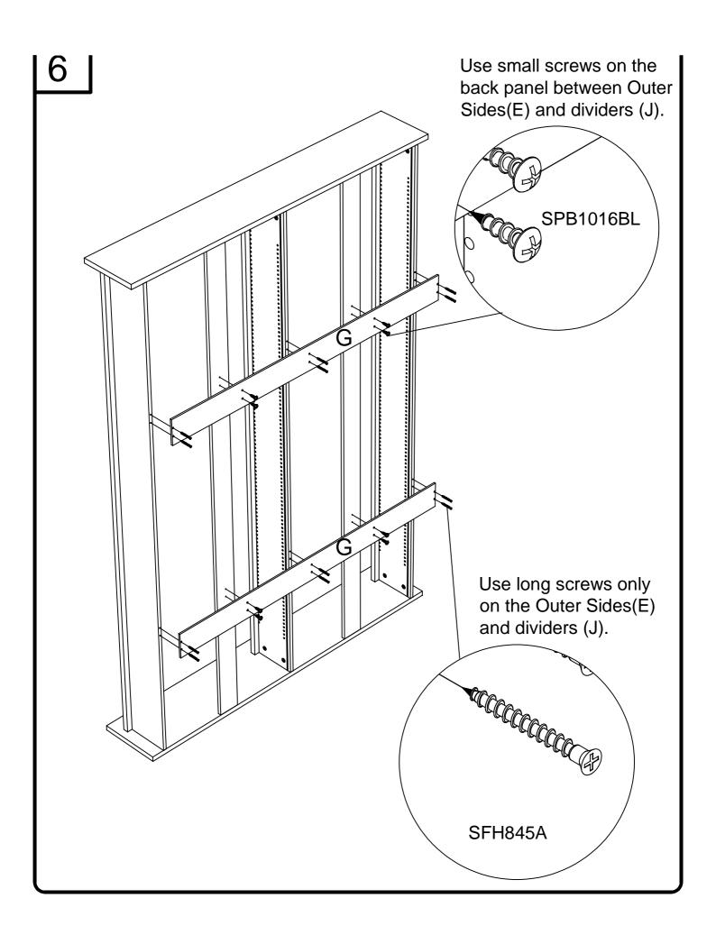
Install Back Panels as snown, with unmarked edges racing down and blue or red marked being atop. Make sure the Blue is on the left side and Red is on the right side of each section. Otherwise you will have problem with leveling of the shelves, they will sag in the middle.
