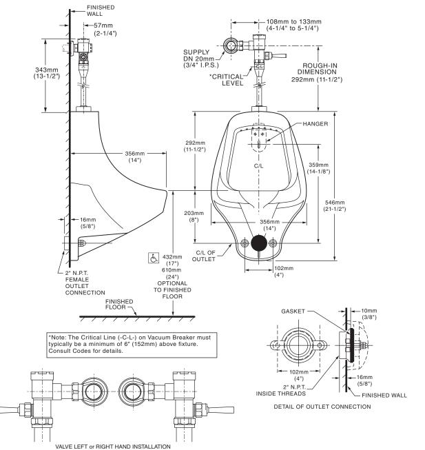
NOTES: PROVIDE SUITABLE REINFORCEMENT FOR ALL WALL SUPPORTS.
