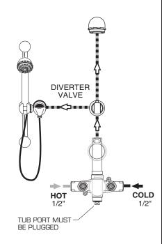
THERMOSTATIC SHOWER INSTALLATION USING A DIVERTER VALVE, FIXED SHOWER HEAD, ADJUSTABLE HAND HELD SHOWER, ON/OFF VALVE AND TWO BODY SPRAYS
