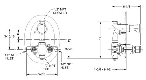
THERMOSTATIC BATH/ SHOWER INSTALLATION USING A TWIN ELL, DIVERTER SPOUT AND FIXED SHOWER
