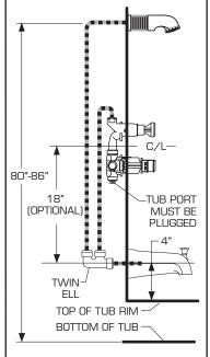
IMPORTANT: WHEN NOT USING A DIVERTER SPOUT A SEPARATE DIVERTER VALVE MUST BE USED. THERMOSTATIC SHOWER INSTALLATION USING A DIVERTER VALVE, FIXED SHOWER HEAD AND ADJUSTABLE HAND HELD SHOWER
