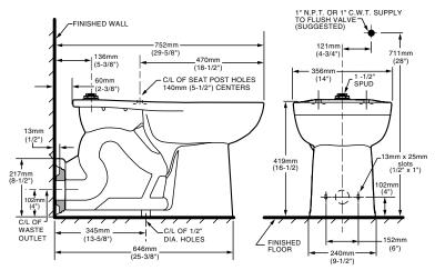
**DIMENSIONS (Nominal)** NOTE: Distance from floor to closet flange centerline (rough-in) must be 4" (102 mm) with flange surface flush to 1/16" (1.6mm) max. beyond finished wall.
