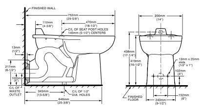
**DIMENSIONS (Nominal)** NOTE: Distance from floor to closet flange centerline (rough-in) must be 4" (102 mm) with flange surface flush to 1/16" (1.6mm) max. beyond finished wall.
