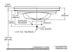
NOTES:  $\star$ DIMENSIONS SHOWN FOR LOCATION OF SUPPLIES AND "P" TRAP ARE SUGGESTED. FITTINGS NOT INCLUDED WITH FIXTURE AND MUST BE ORDERED SEPARATELY. FOR COUNTERTOP CUTOUT AND INSTALLATION INSTRUCTIONS USE TEMPLATE SUP-
