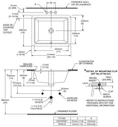
WE RECOMMEND USING BASIN AS A TEMPLATE TO DETERMINE PROPER CONTOUR. CUT COUNTERTOP 38MM (1-1/2") INSIDE BASIN CONTOUR.
