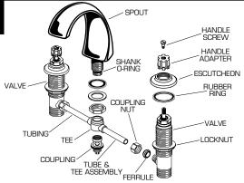
VALVE inlet is 3/4-inch NPT male connector.
