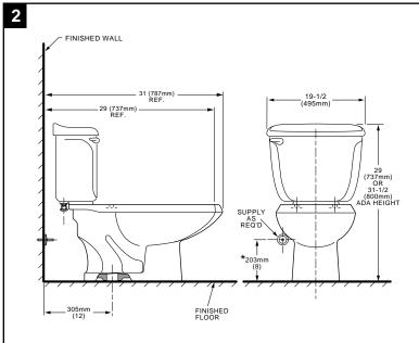
**DIMENSIONS (Nominal)** NOTE: Distance from wall to closet flange centerline (rough-in) must be 12" (305 mm) minimum.
