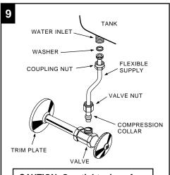
CAUTION: Overtightening of COUPLING NUT could result in breakage and potential flooding.
