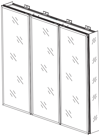
SURFACE MOUNTED CABINET SHOWN
