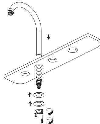
2. Position the spout shank in the second hole of sink. Secure with rubber seal, metal washer, and tighten the spout shank with lock nut.
