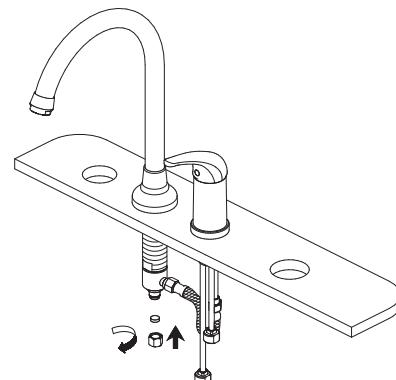
5. Connect thread pipe of handle body and spout shank with hose.
