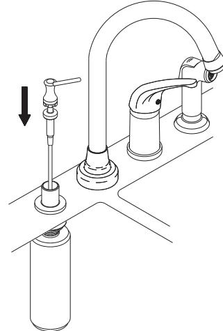
**18.** Re-assemble the chrome pump nozzle and plastic pump onto connector.
