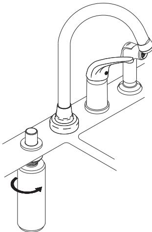
**16.** Insert the bottle and tighten with lock nut.
