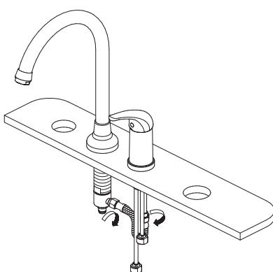
4. Place the body in the third hole of sink. From underneath the sink, replace the washer and lock nut.
