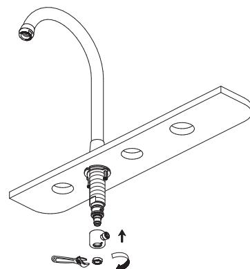
3. Install adaptor to the spout shank and secure with the nut to fix up.
