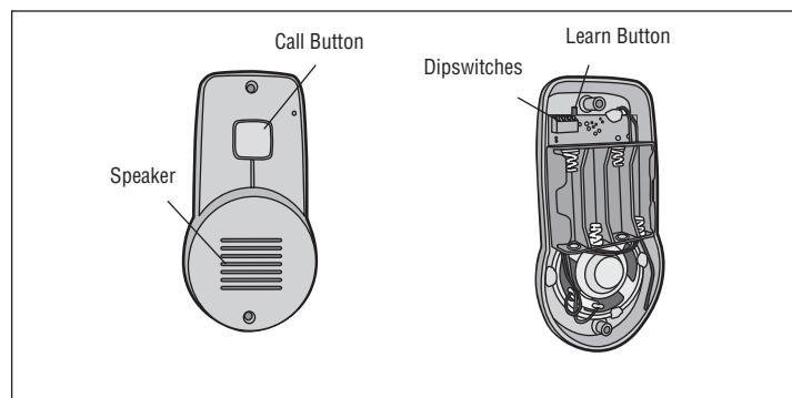
**Call Button:** To make a call, press and release the call button and all intercoms in the network will receive the signal. When the call is answered by an intercom, a secure channel is created between the two and the other intercoms in the network do not hear the conversation. Once a secure connection is made, the call button on the doorbell does not need to be pressed to speak.
