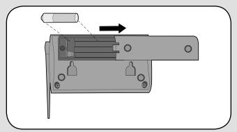
Install 4 AA Alkaline batteries (not provided).
