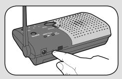
Before programming, clear memory on all intercoms. Press the Learn button on the new intercom until a beep is heard. Within 10 seconds put the second intercom into Learn Mode (refer to the following table).
