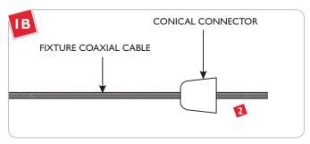
Insert the fixture coaxial cable through the conical connector.
