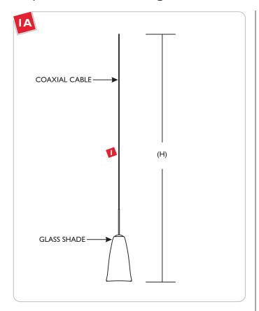
• Cut the coaxial cable to the desired length with a sharp cutter. The overall fixture height (H) is measured from bottom of the glass shade to the end of the coaxial cable.
