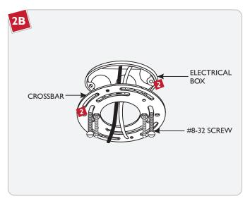
Mount the crossbar to the electrical box with two #8-32 screws.
