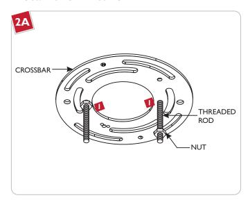
Screw one nut onto each threaded rod and tighten it to secure the threaded rod in place.
