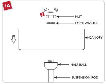
1 Attach the canopy to the suspension rod by placing it on the half ball and securing it with the lock washer and nut.
