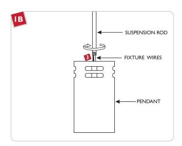
3 Feed the fixture wires through the suspension rod and screw the suspension rod into the pendant.
