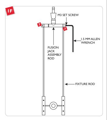
Insert the fixture rods into the Fusion Jack assembly rod, make sure the fixture rods are aligned with the top of the Fusion Jack assembly rod. Tighten the two M3 set screw with 1.5 MM Allen wrench.
