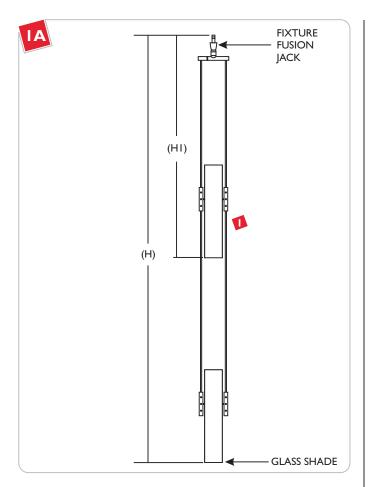
The overall fixture height (H) is measured from bottom of the bottom glass shade to the end of the fixture Fusion Jack.
