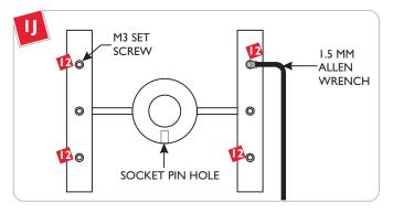
Loosen (**Do Not Remove**) the four M3 set screws on the middle socket assembly rods.
