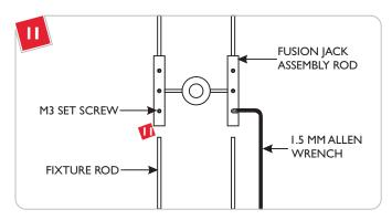
Insert the fixture rods into the top Fusion Jack assembly rods, and tighten the two M3 set screw with 1.5 MM Allen wrench.
