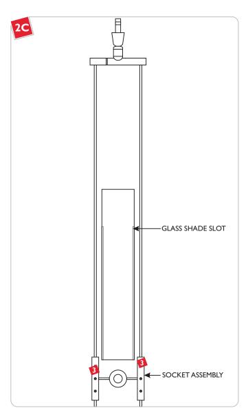
From between the fixture rods, carefully place a glass shade onto each socket assembly.
