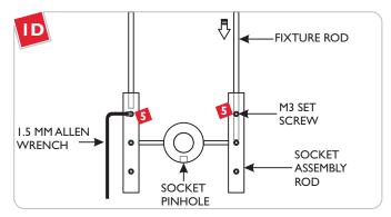
Insert the two fixture rods on the opposite side of socket pin holes, completely into the socket assembly rod and secure into place by tightening the M3 set screws with the provided 1.5 MM Allen wrench.
