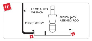
Loosen (**Do Not Remove**) the two M3 set screws on the sides of the Fusion Jack assembly rod with the provided 1.5 MM Allen Wrench.
