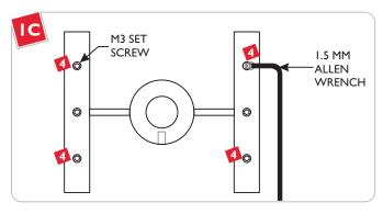
Loosen (**Do Not Remove**) the four M3 set screws on the socket assembly rods.
