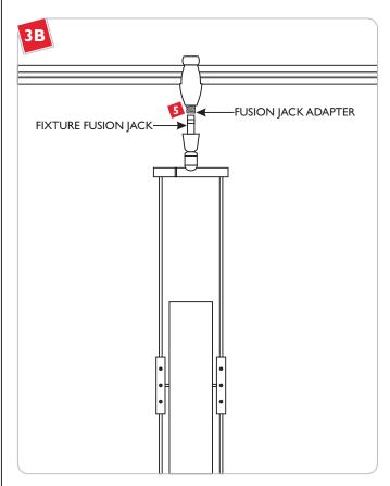
Push and screw the fixture Fusion Jack completely into the Fusion Jack adapter.
