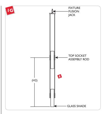
The height (H2) is measured from bottom of the bottom glass shade to the middle of the top socket assembly rods.
