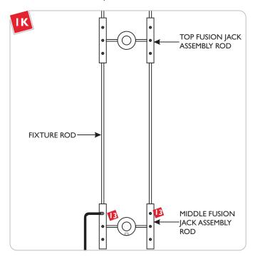
Insert the Fusion Jack assembly rods from the end opposing the socket pin holes onto the fixture rods. Make sure that the bottom Fusion Jack assembly rods are in line with the top Fusion Jack assembly rods and tighten the two M3 set screws with the 1.5 MM Allen wrench.
