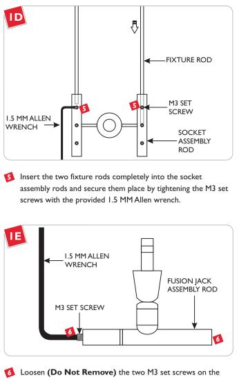
Loosen (Do Not Remove) the two M3 set screws on the sides of the Fusion Jack assembly rod with the provided I.5 MM Allen wrench.
