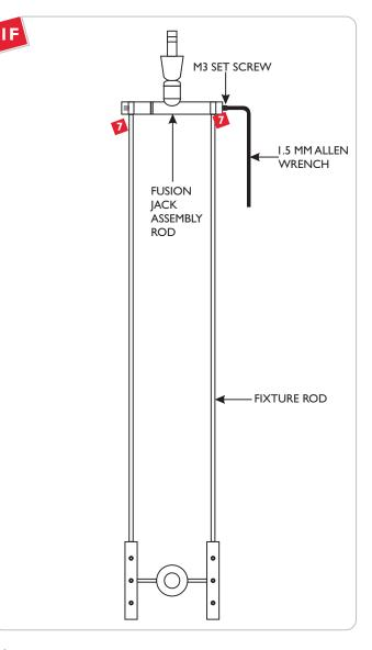
Insert the fixture rods into the Fusion Jack assembly rod, make sure the fixture rods are aligned with the top of the Fusion Jack assembly rod. Tighten the two M3 set screw with 1.5 MM Allen wrench.
