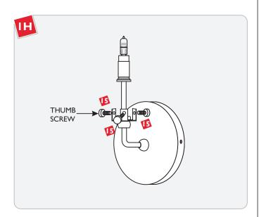
Remove the three thumb screw.
