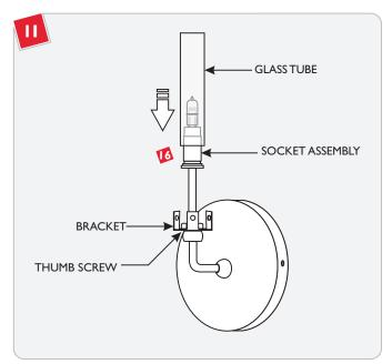
Carefully slide the glass tube ono the socket assembly.
