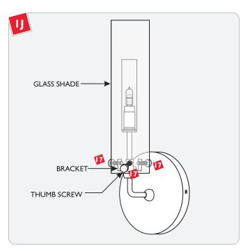
Align the glass holes with the bracket holes. Replace and tighten the three thumb screws to secure the glass shade in place.
