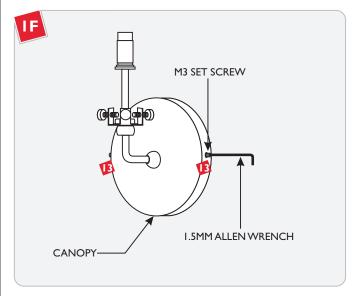
Place the fixture canopy onto the backplate. Level the fixture vertically and tighten the two M3 set screws with the 1.5MM Allen wrench to secure the fixture in place.
